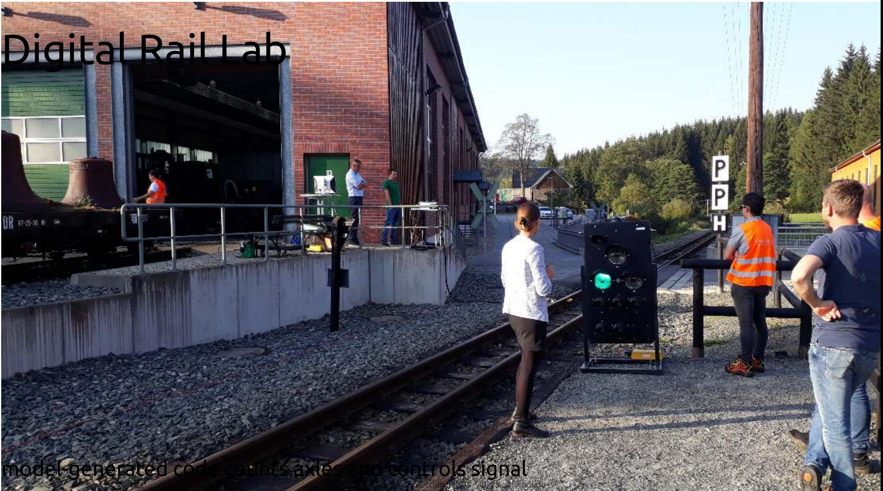
model-generated code counts axles and controls signal
